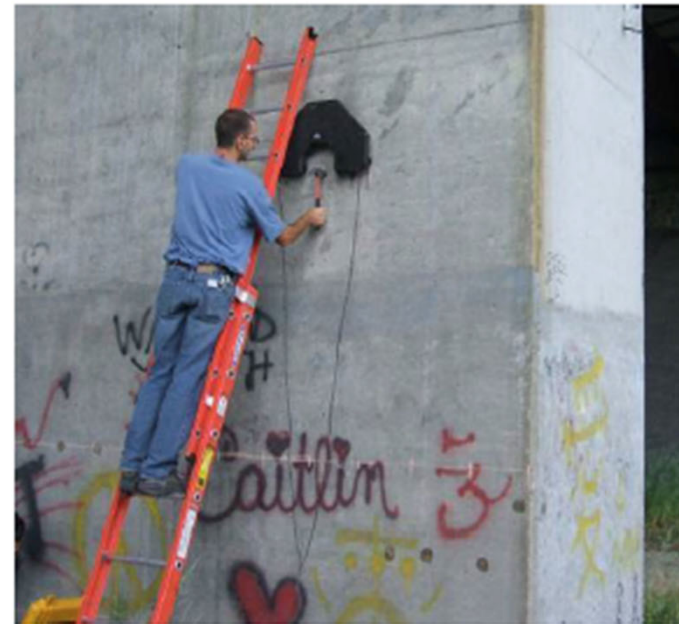
A. Impact-echo B. Non-Linear acoustic technique
