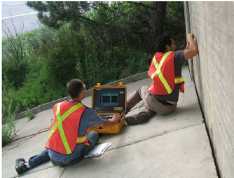
A. Impact-echo B. Non-Linear acoustic technique
